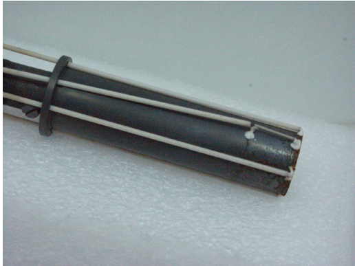
Photo 1: sample with thermocouples
